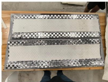
Figure 14. Two layers of carbon and core before laminating (Krušvar, 2024)
