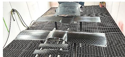
Figure 17. Coating of the produced elements (Krušvar, 2024)
