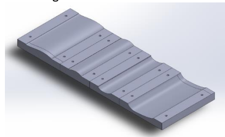
Figure 12. Profile fabrication molds (Krušvar, 2024)
