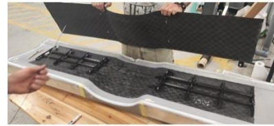
Figure 16. Assembly and reinforcement of the front spoiler (Krušvar, 2024)
